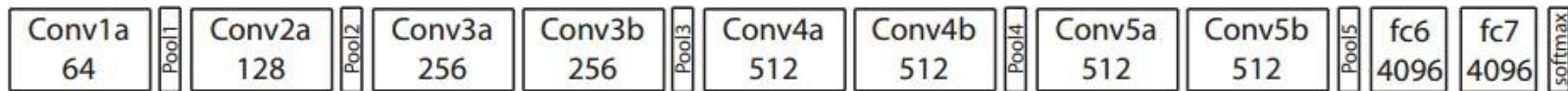
Figure 3. C3D architecture. C3D net has 8 convolution, 5 max-pooling, and 2 fully connected layers, followed by a softmax output layer. All 3D convolution kernels are 3 \times 3 \times 3 with stride 1 in both spatial and temporal dimensions. Number of filters are denoted in each box. The 3D pooling layers are denoted from pool1 to pool5. All pooling kernels are 2 \times 2 \times 2 , except for pool1 is 1 \times 2 \times 2 . Each fully connected layer has 4096 output units.
