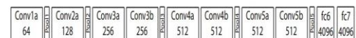
Figure 3. C3D architecture. C3D net has 8 convolution, 5 max-pooling, and 2 fully connected layers, followed by a softmax output layer. All 3D convolution kernels are 3 \times 3 \times 3 with stride 1 in both spatial and temporal dimensions. Number of filters are denoted in each box. The 3D pooling layers are denoted from pool1 to pool5. All pooling kernels are 2 \times 2 \times 2 , except for pool1 is 1 \times 2 \times 2 . Each fully connected layer has 4096 output units.
